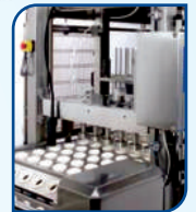
Finished Product ejection station
