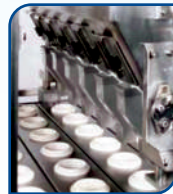
Chopped nuts distribution station
